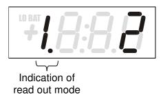
While the address unit is in read out mode the stored short address can be read out of the device by pressing button "Enter". After read out the stored short address is displayed on the LCD.
