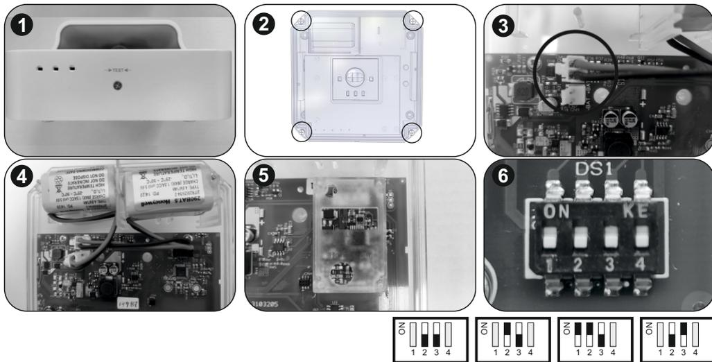
**Step 1:** Unfasten the front screw and remove the cover.
