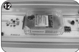
The device comes with 4 label stickers that contain a Unique identification code (UID) that is hexadecimal formatted in 4 bytes. An example UID is **45 90 DB FA**. It is advised to stick one sticker on the module and one sticker on the luminaire that the module will be fitted in. The two remaining stickers may be placed on a printed floor plan, text lists etc.
