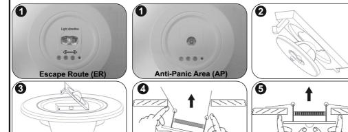
Step 1: In order to place the proper lens (Anti - panic or escape route), first be sure that the luminary is not connected in the mains power supply and the battery is disconnected. A 5 lux lens (Part no. 2900XX.STR) is also available for order. Use the corresponding lens retaining cover depending on the lens you will use.
