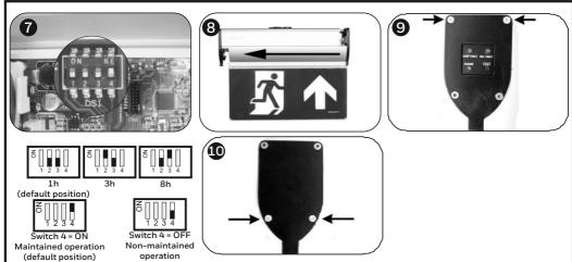
**Step 7**: The control of maintained or non maintained operation of the luminary is achieved through Switch 4 of DS1. For maintained operation, switch number 4 must be in ON position. For non-maintained operation, switch number 4 must be in OFF position.
