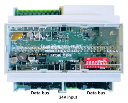
Relay with status LEDs 3 yellow LEDs inform about the status of the data bus
