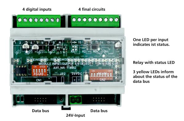
**Functionality** Each circuit can be controlled from a higher level or from external switching inputs. Several types of fuse are possible for the protection of the circuits, which are permitted according to the regulations. Via external potential-free contacts, each of the four 24 VDC inputs can be assigned to one or more circuits of the safety lighting system.
