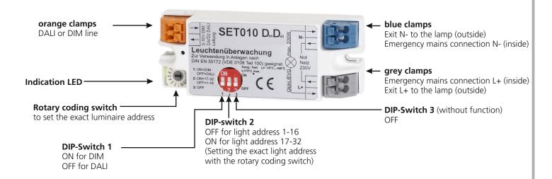
**Functionality** Deactivation of the DALI or DIM control in test and emergency mode and switching on of any luminaire in the circuit (= select circuit) To ensure that the DALI luminaires switch back to the desired state as quickly as possible after completion of the test or emergency mode, we recommend programming a short repetition time of the DALI control command (this programming is done via the individually used DALI control).
