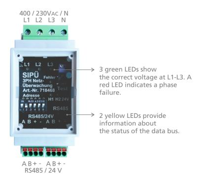
**Funktionality** This bus mains monitor is system-bound and communicates directly with systems of the BUSINESS series. It is equipped with a safety function: The communication monitoring reacts to line interruption or short-circuit; a fault is reported in the event of communication errors.
