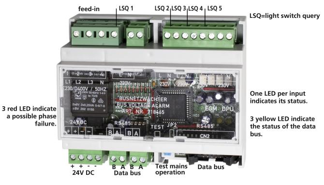
**Function** This bus mains monitor is system-bound and communicates directly with the emergency lighting system. It is equipped with a safety function: The communications monitor reacts to breakages or short-circuits in the cable; a fault is reported when communication errors occur.
