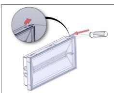
**Step 1:** Pull up gently the diffusor's clips from both sides to remove the diffusor.
