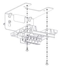
**Step 2:** Install the socket to the metallic base and fasten the two supplied screws.
