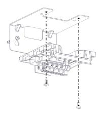
Step 2: In stall the socket to the metallic base and fasten the two supplied screws.
