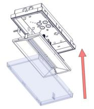
**Step 6:** Refit carefully the removed parts (Step 1 & 2). The diffusor must be secured (click sound). This requirement is important to ensure the IP65 rating.
