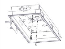
**Step 5:** Install the ImPerLED base to the metallic base and fasten the 2 supplied screws with the 2 sealing o-rings.
