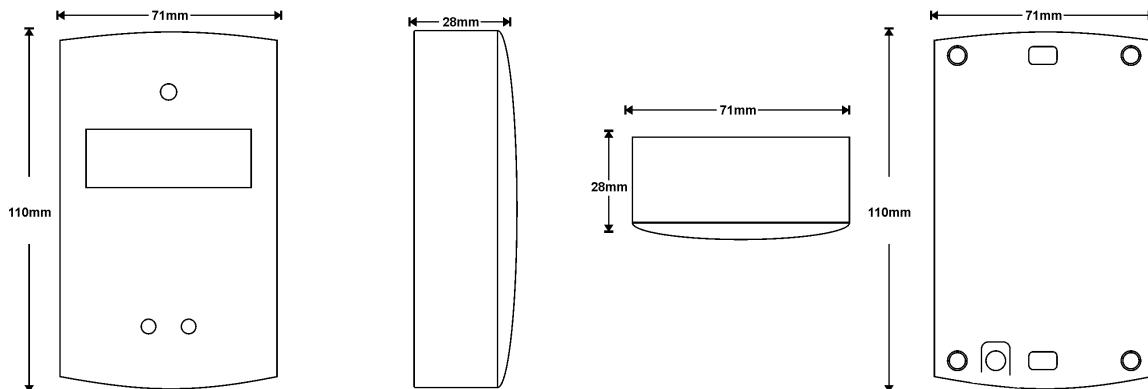
This handheld device gives the ability to check the received signal strength (RSSI) on any position of the installation area, in order to optimize the communication quality of the network.
